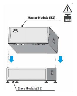
4. Remove the front covers of B2 and B1. When removing the front cover of B2, disconnect the cable behind the Start/ Stop button first.
