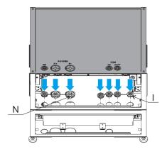
6. Use the bonding strips to fix B1 and B2 with screws M5×14.(Torque, 4.5 Nm)
