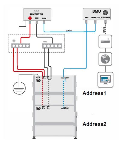
The battery system connected to BMU is appointed as Address 1, and the battery system connected to Address 1 is appointed as Address 2.
