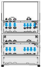
13. Fix B2 and B1 in both two battery systems and between B2 (the first battery system) and B1 (the second battery system) with six bonding strips.
