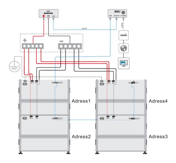
The battery system connected to Address 2 is appointed as Address 3, and so on.
