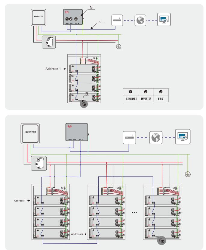
The connection to an Ethernet cable is recommended, not compulsory.
