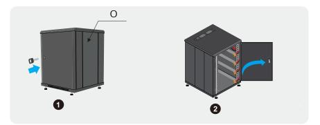
Put the modules into the dedicated positions of the cabinet. Install the screw and fasten the modules to the cabinet. (torque: 5.5 ± 0.5 Nm)
